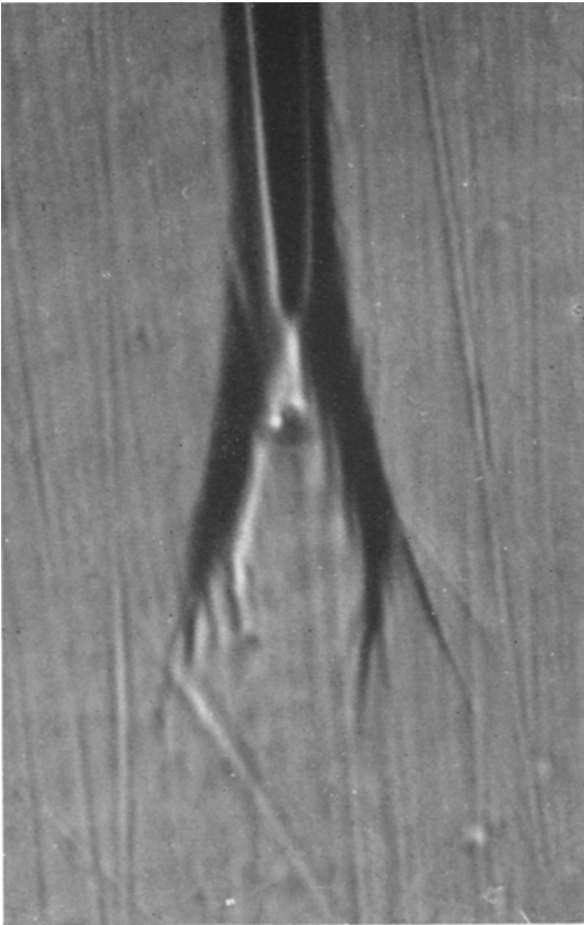
Figure 9 Blunt crack tip in a sample sheet of Araldite with 15 pph hardener ( \times 2200 ).
